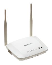
THE SR360n DSL GATEWAY provides high performance and flexibility for broadband and IPTV subscribers. It combines a full-rate ADSL modem with a wireless access point using the latest 802.11n WiFi technology. It can be used as an Ethernet or DSL gateway, and includes a router, firewall, and TR-069 management.
